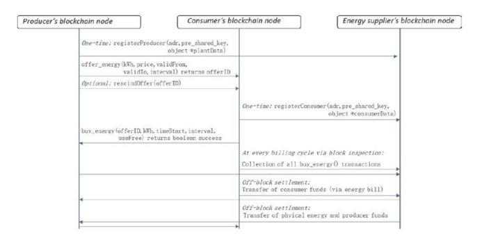
Figure 13: Technical flow of Lition energy transactions
